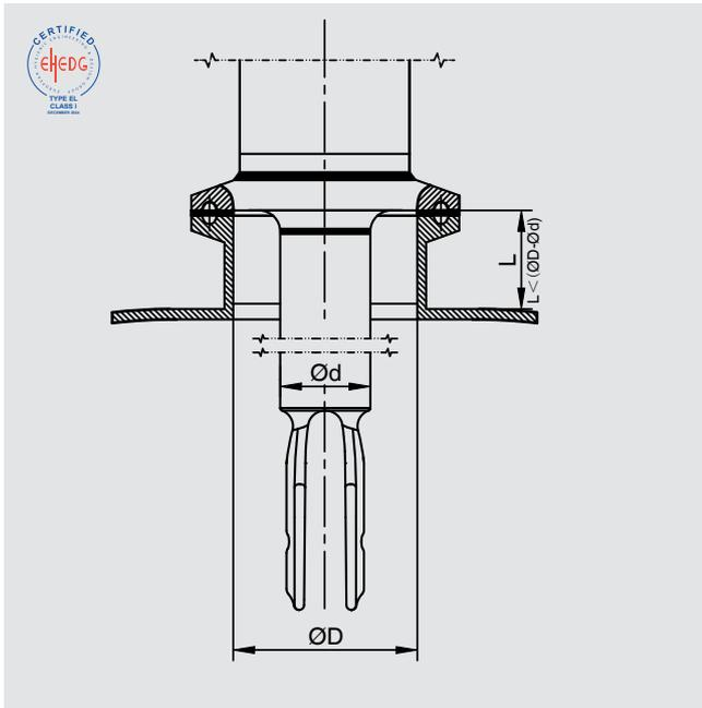
Sensors inserted in tanks should be flush with the inside of the tank wall. If, for technical reasons, there is a dead space, it must be ensured that the spray jet from the cleaning appliance can reach all surfaces. To fulfil the EHEDG cleaning criteria, the maximum length of the tank nozzle,  $L_{\max}$ , should be taken into account.
