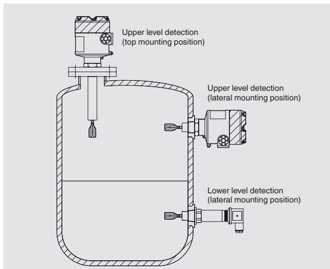
The vibrating level switch is usually installed on the side of the tank to detect the upper and lower liquid level. If the vessel has no side openings, the level switch can also be mounted on the tank from above. A pipe extension is then often used to achieve the desired switch point. Installation on the bottom of the tank is also possible.
