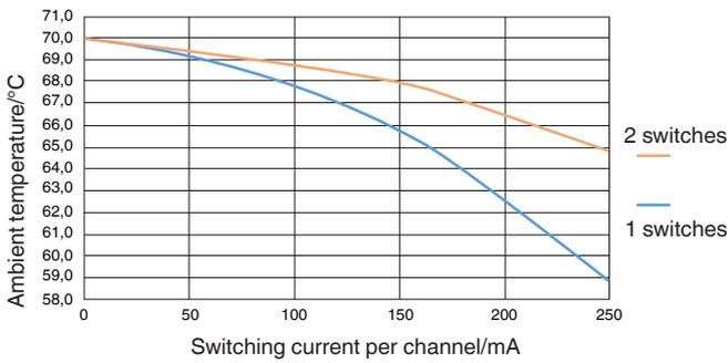
Max. ambient temperature, if medium temperature = 85 °C [185 °F]
