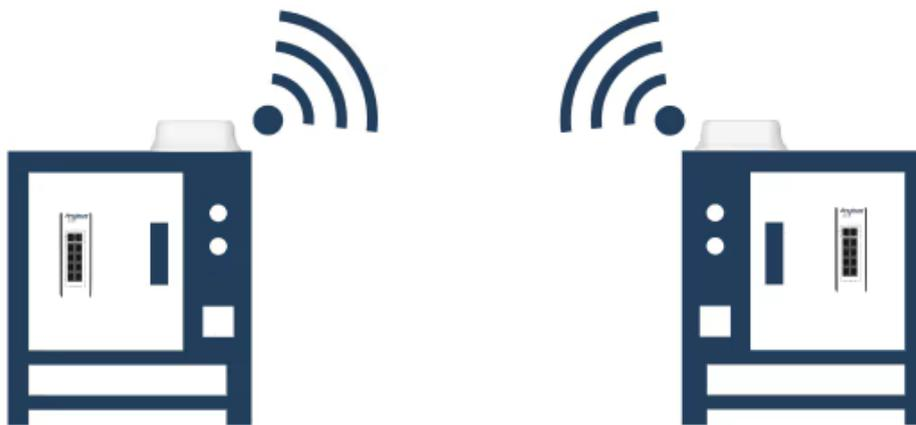
The Anybus Wireless Bolt II is configured as an access point and mounted on a cabinet to allow wireless access between an HMI and the equipment in the cabinet. The Bolt II is powered by a PoE switch inside the cabinet.
