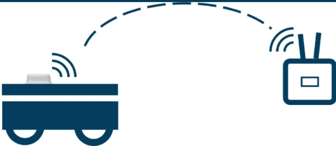
The Anybus Wireless Bolt II can be attached to roaming machines such as AGVs, enabling the machine to connect to various access points throughout the facility. It exchanges information on the best path to ensure the machine reaches its destination efficiently and safely.
