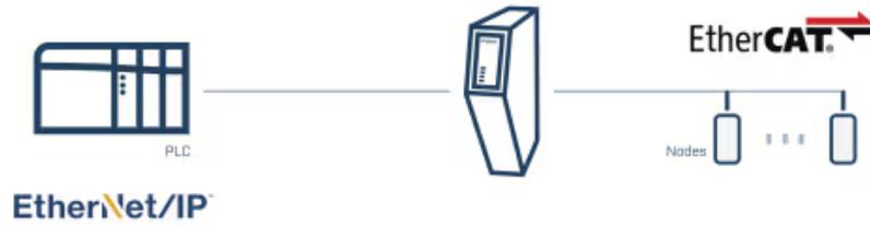
The communicator can be used wherever there is a need to transfer data between control systems using different industrial protocols.
