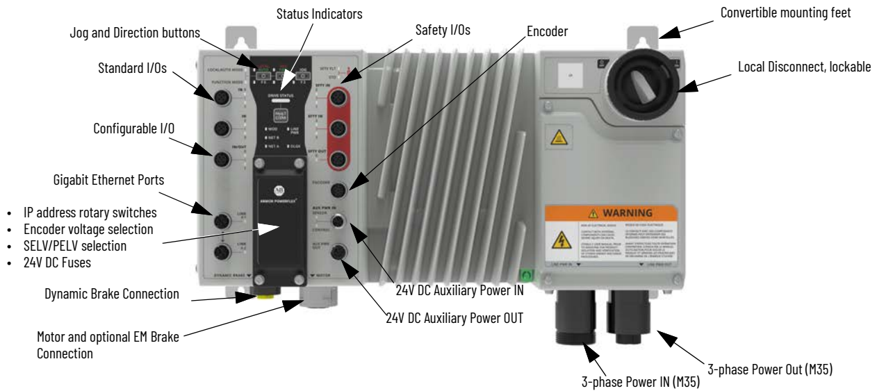
Figure 2 - Armor PowerFlex AC Drive Features, Frame B (shown: Drive with integrated safety version, with external power supply)
