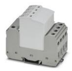
Plug-in surge arrester, in accordance with Type 2/Class II, for 3-phase power supply networks with separate N and PE (5-conductor system: L1, L2, L3, N, PE), with remote indication contact.
