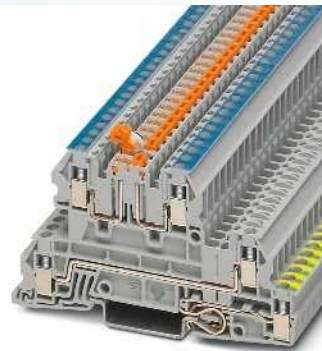
4 (4) mm 2 , 24 A, three-level terminal block, 1 x L phase conductor, 1 x N conductor can be disconnected, 1 x PE
