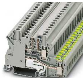
0.5 A, diode terminal block, 1N 4007 (1300 V/0.5 A), conducting direction: from left to right
