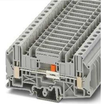
50 A, measuring transducer disconnect terminal block, 4 plug-in bridge shafts, 2 screw bridge shafts
