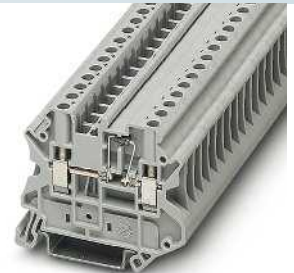
0.5 A, diode terminal block, 1N 4007 (1300 V/0.5 A)
