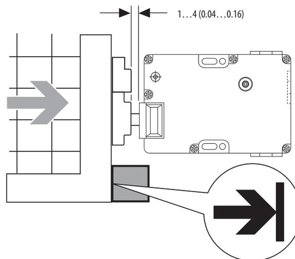
As shown in [Figure 11](#), the TLSZ has two slotted holes to facilitate installation. The slots allow up to 8 mm (0.31 in.) of movement of the switch body to achieve the proper clearance with the actuator.
