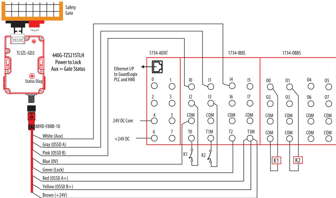
Figure 24 shows the General Tab of the 1734-IB8S Module Properties. The Input Status must be set to “Combined Status – Muting” as this setting is used by the Dual Channel Input Stop logic block to verify that 1734-IB8S is operational. The Output Data must be set to “Test,” as the test outputs are used to generate test pulses for the output contactors.
