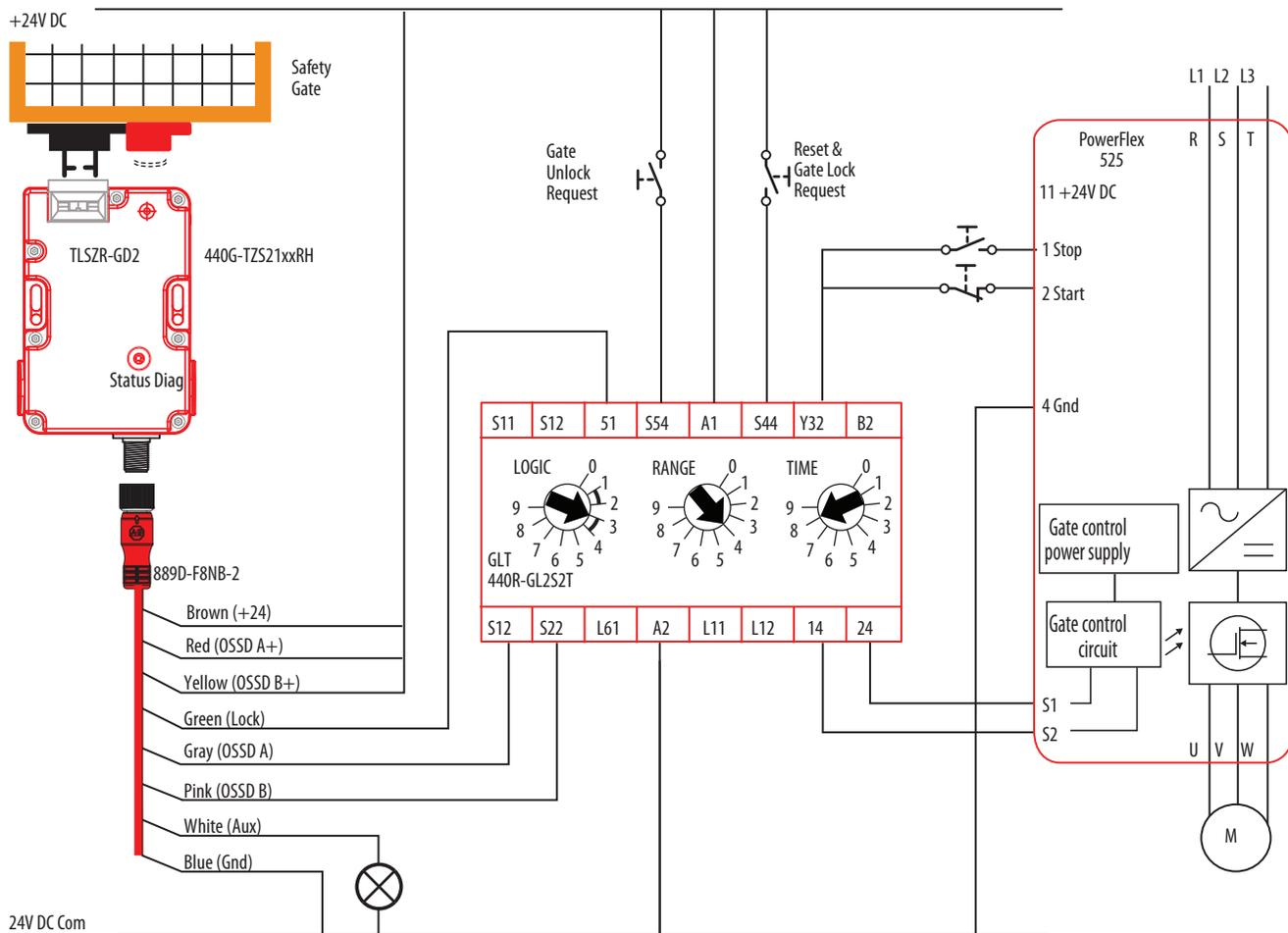
Circuit status as shown: The gate is open and unlocked. The motor is off. The GLT is ready for reset. The GLT has a Logic setting of 3: (Category 1 Stop), a Range setting of 4 (10 seconds) and a Time setting of 8 (80%). The Y32 output turns OFF immediately; 8 seconds later, the safety outputs turn OFF.
