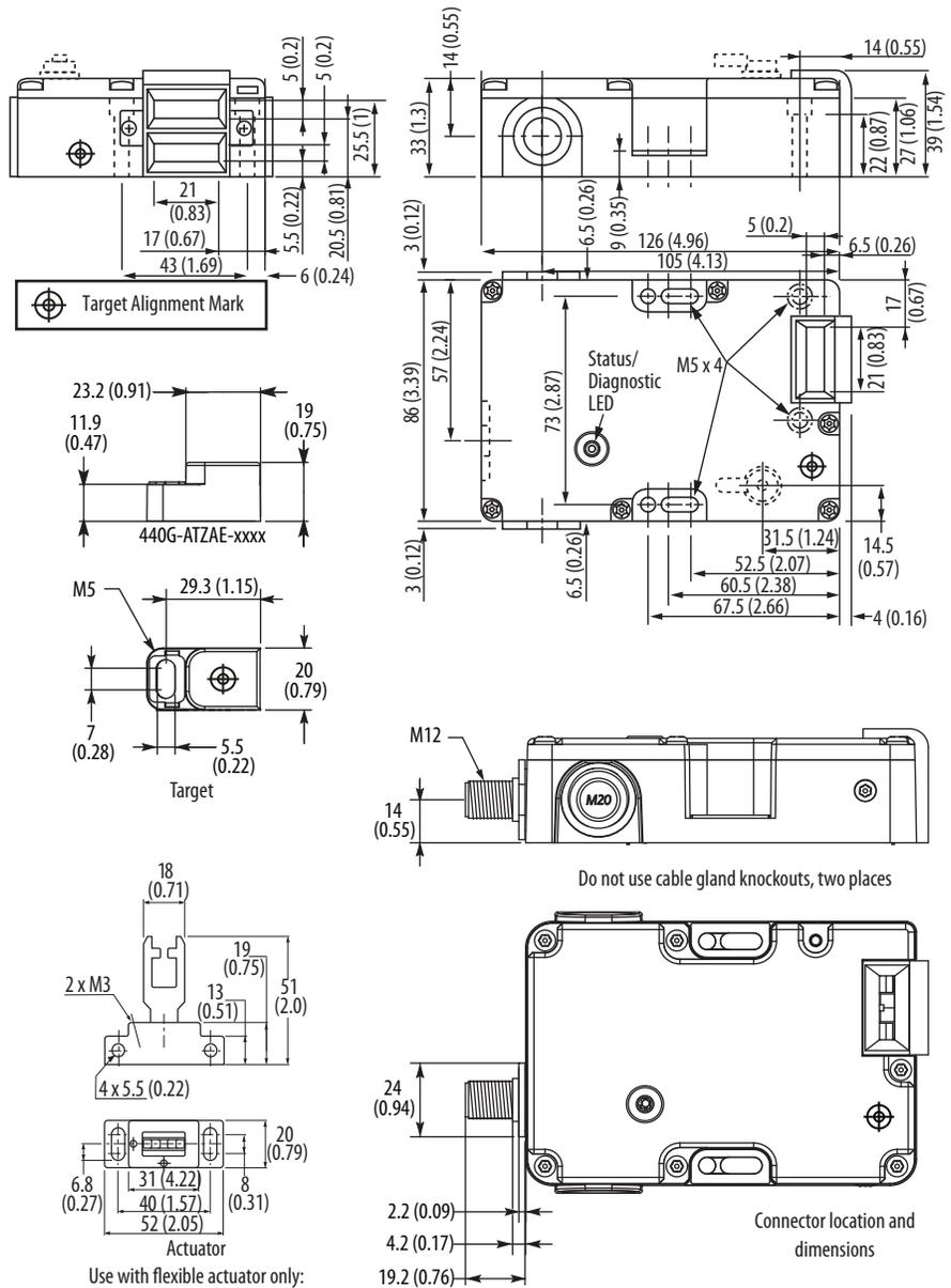
Figure 13 on page 18 shows the dimensions for mounting the target that is next to the actuator.
