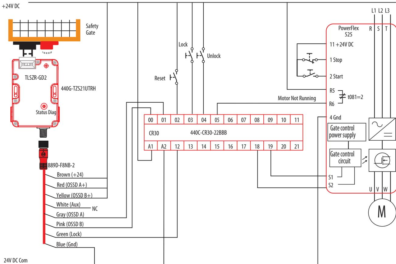
Figure 22 on page 34 shows an example CR30 configuration that works with the schematic in Figure 21.
