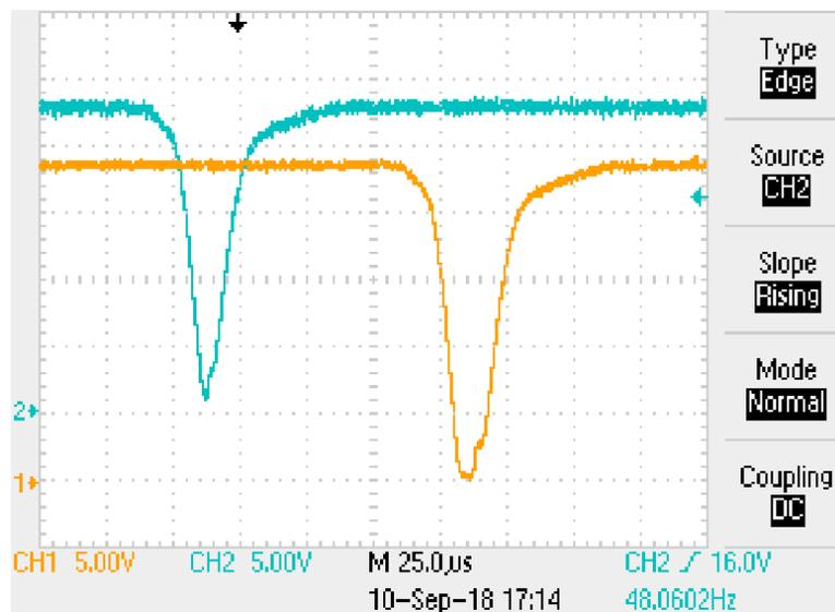
In Figure 41 on page 49, a TLSZR and GSR-SI operate successfully with long wiring. The OSSD outputs drop to approximately 21V and the test pulses only drop to approximately 8V (not 0V).
