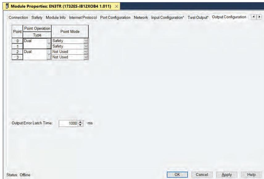
Figure 35 shows an example program. A Dual Channel Input Stop function block monitors the TLSZR and a Configurable Redundant Output function block controls two contactors. This example can be used as a starting point for implementation; based on the risk assessment for the machine, you can incorporate additional logic.
