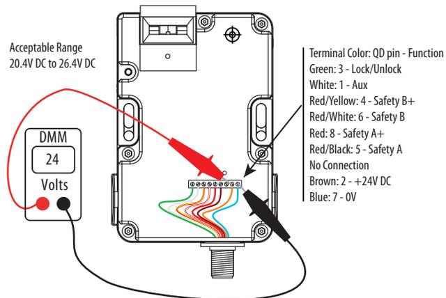
If 24V is present at the wiring terminals, then check that the wires are stripped and the terminal screws are tight. If the wires are okay, then replace the switch.
