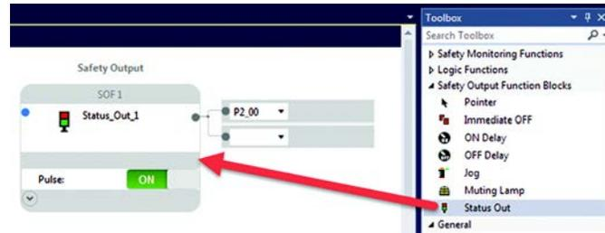
See [Figure 74 \(page 76\)](#) and [Figure 75 \(page 77\)](#) for examples of how the Status Out block works with the Status In block. [Figure 73 \(page 76\)](#) shows how the Status Out block is used with other functions. In this example, the Status\_Out\_1 block pulses its output as soon as the E-stop button is pressed. When the E-stop button is released, the Status\_Out\_1 block turns OFF.
