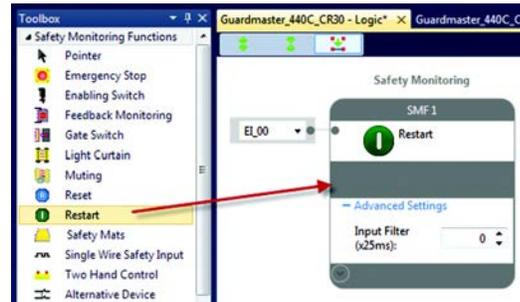
The Restart Function requires a leading and trailing edge within a specific time frame. The pulse width must be between 250...3000 ms. If the pulse width is too short or too long, the Restart function is not executed.
