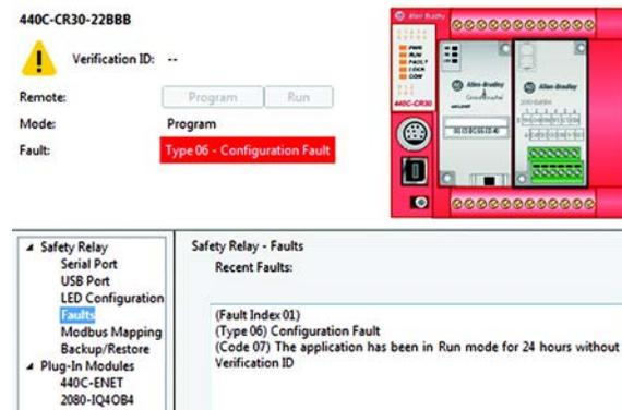
If the safety system is verified, the CR30 safety relay assigns a four-digit number and allows the relay to operate in Run mode beyond the 24-hour limit. After verification, the Run status indicator remains solid green.
