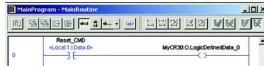
The signal can be used within the safety relay logic by selecting the corresponding Communications Input selection from a Safety Monitoring Function that supports standard rated signals.
