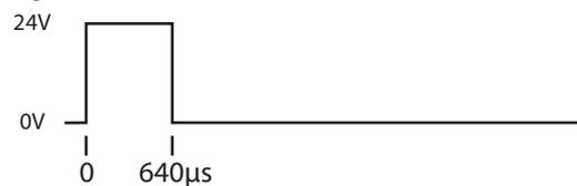
When multiple terminals are configured for normally open operation, the CR30 safety relay tests each one at 500-ms intervals. This test sequence is repeated every 6.4 seconds.
