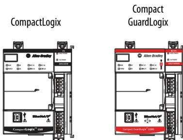
When you configure your CompactLogix 5380 or Compact GuardLogix 5380 control system, you must account for the number of EtherNet/IP nodes that you include in the I/O configuration section of your project.
