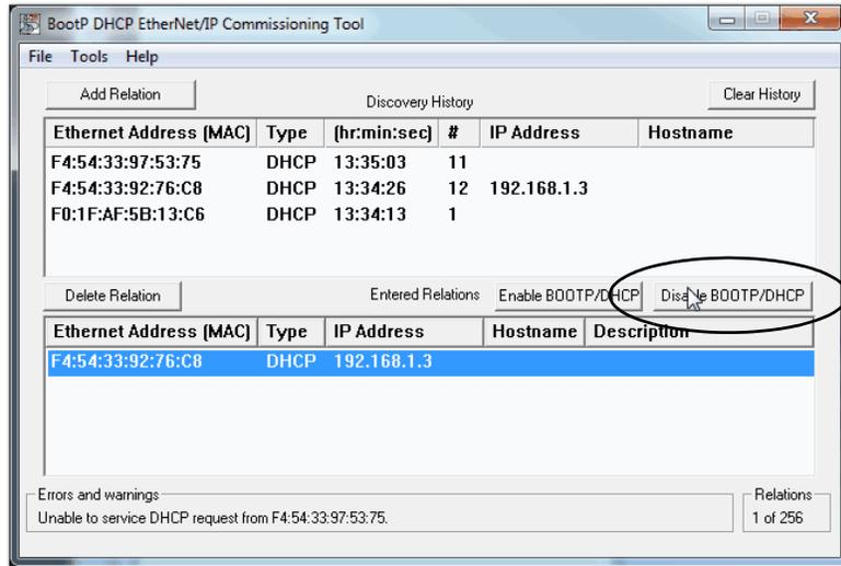
The module now uses the assigned configuration and does not issue BOOTP or DHCP requests after power is cycled on the controller.
