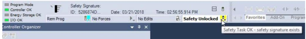
The Safety Status button itself indicates whether the controller is safety-locked or -unlocked, or faulted. It also displays an icon that shows the safety status.
