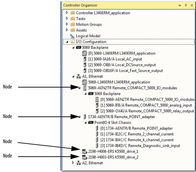
The Capacity tab in the Controller Properties dialog box displays the number of Ethernet nodes that are used in a project. The following graphic is representative of the project shown in Figure 21.
