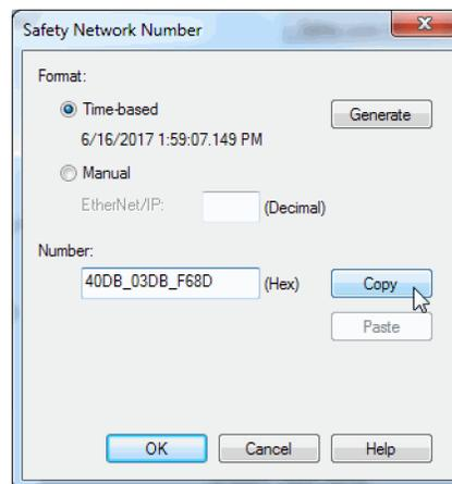
**TIP** You can also copy the SNN directly from the Safety Tab. On the Safety tab, select the cell with the SNN. Right-click and select Copy (or press Ctrl-C).
