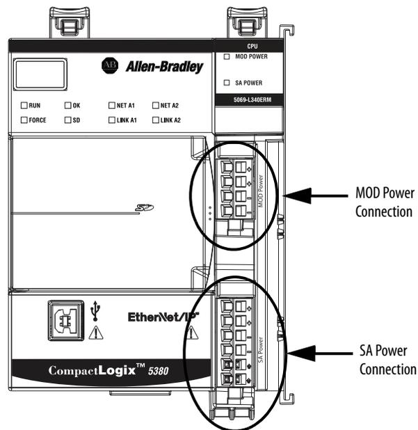
Power begins at the controller and passes across the Compact 5000 I/O module internal circuitry via power buses.
