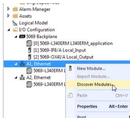
The Logix Designer application automatically detects available modules that are installed in the system.
