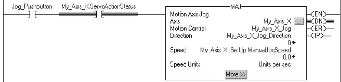
If Jog\_Pushbutton = off, the MAS instruction stops the axis at 100 units/second<sup>2</sup>. Make sure that Change Decel is Yes. Otherwise, the axis decelerates at its maximum speed.
