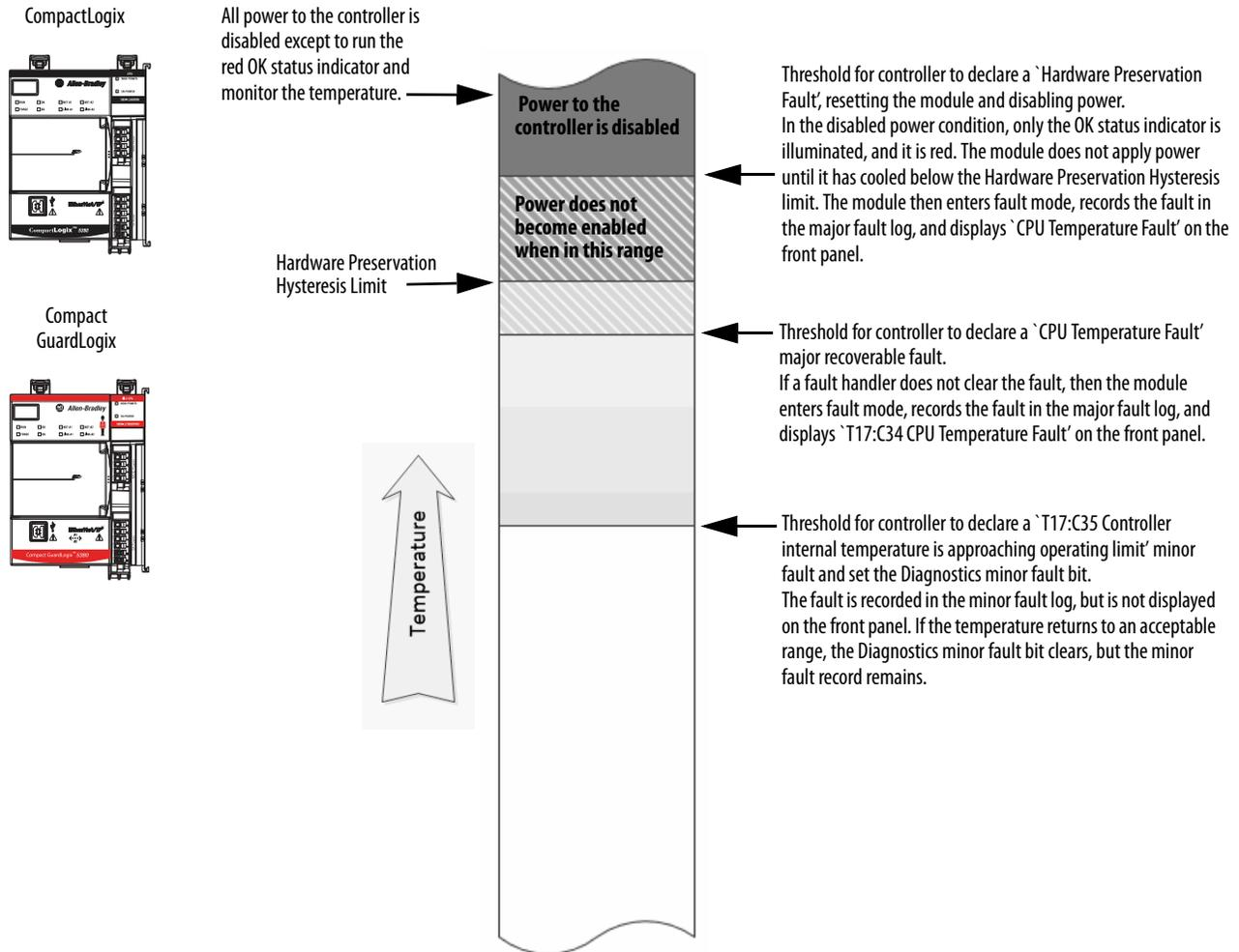
**IMPORTANT** If you follow the recommended limits for ambient (inlet) temperature and apply the required clearances around the system, the controller is unlikely to reach the initial warning (minor fault) temperature.
