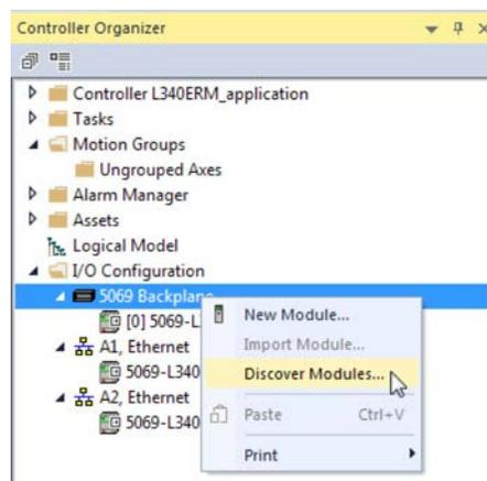
The Logix Designer application automatically detects available modules that are installed in the system.
