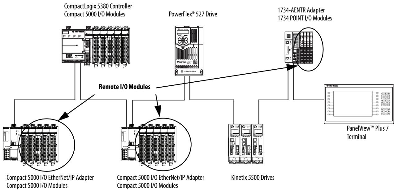
Figure 34 - Remote I/O Modules in a CompactLogix 5380 System on a Star Network Topology
