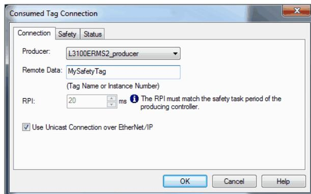
5. From the Producer pull-down menus, select the controller that produces the data.
