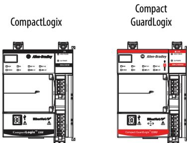
The controllers let you produce (transmit) and consume (receive) controller-scoped tags. CompactLogix™ 5380 and Compact GuardLogix® 5380 controllers produce the same standard tag through the Ethernet ports and the backplane, and consumer counts apply to the total consumers from all ports.
