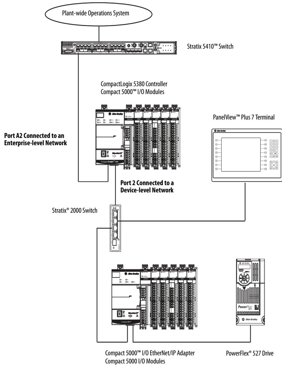
Figure 26 shows a CompactLogix 5380 controller using Dual-IP mode in with connections to separate device-level networks, including a DLR network.
