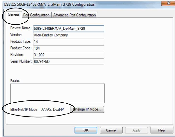
You set the IP Address and Network Mask on the Port Configuration tab.
