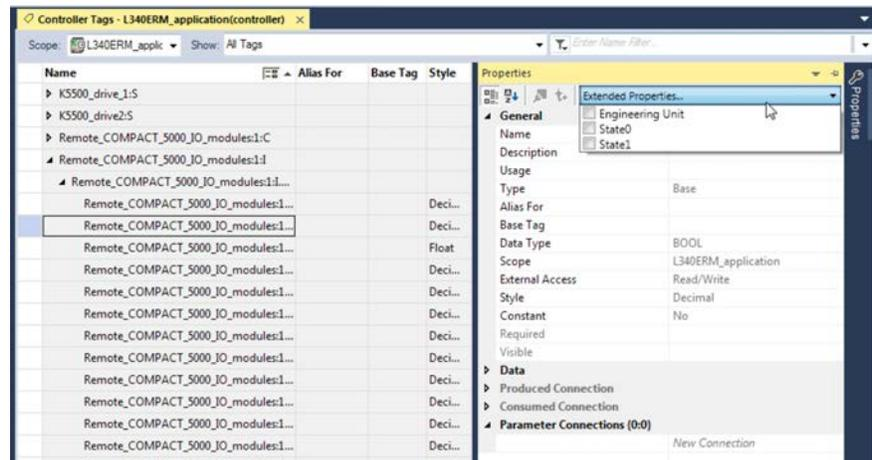
Pass-through behavior is the ability to assign extended properties at a higher level of a structure or Add-On Instruction and have that extended property automatically available for all members. Pass-through behavior is available for descriptions, state identifiers, and engineering units and you can configure it.
