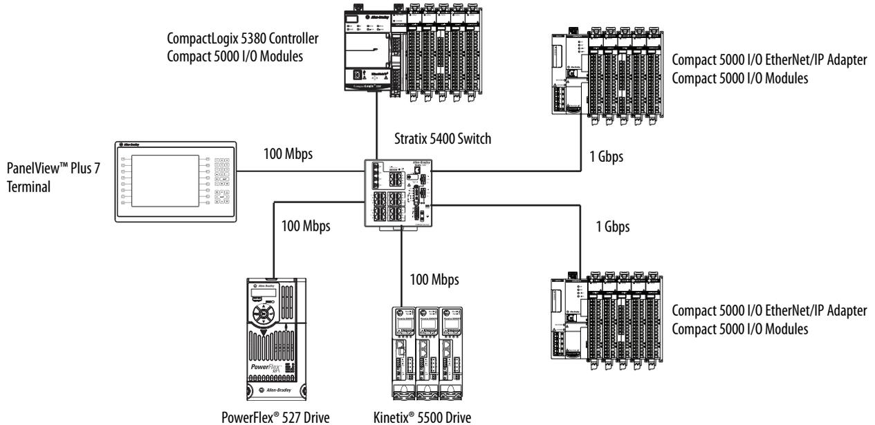
We recommend that you do not use the 1 Gbps network communication rate on the controller ports if it operates on a linear or DLR network topology and at least one device on the network supports the maximum network communication rate of 100 Mbps.
