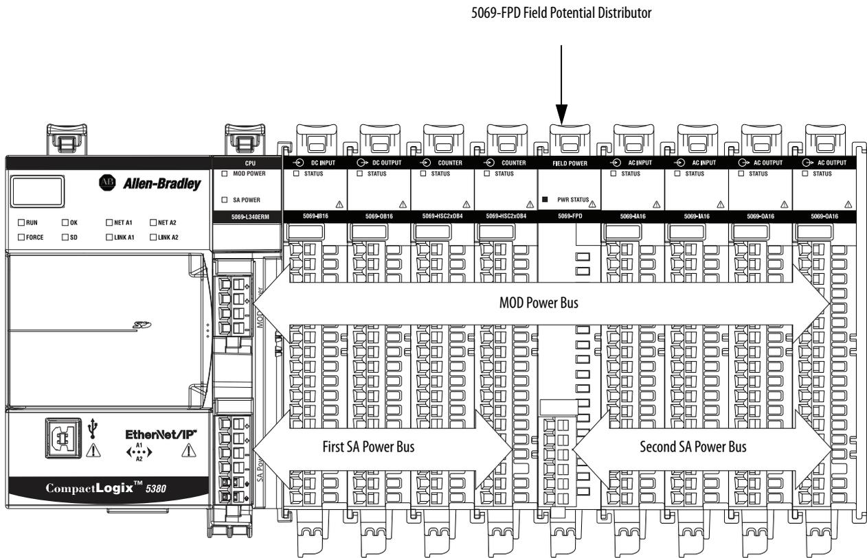
You can install multiple 5069-FPD field potential distributors in the same system, if necessary.
