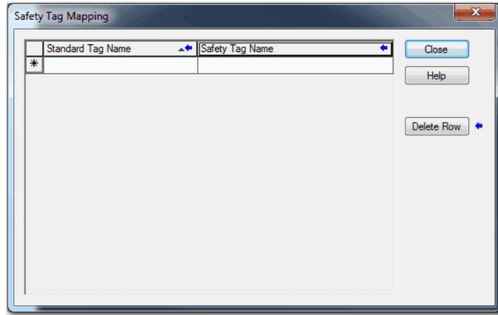
2. Add an existing tag to the Standard Tag Name or Safety Tag Name column by typing the tag name into the cell, or choose a tag from the pull-down menu.
