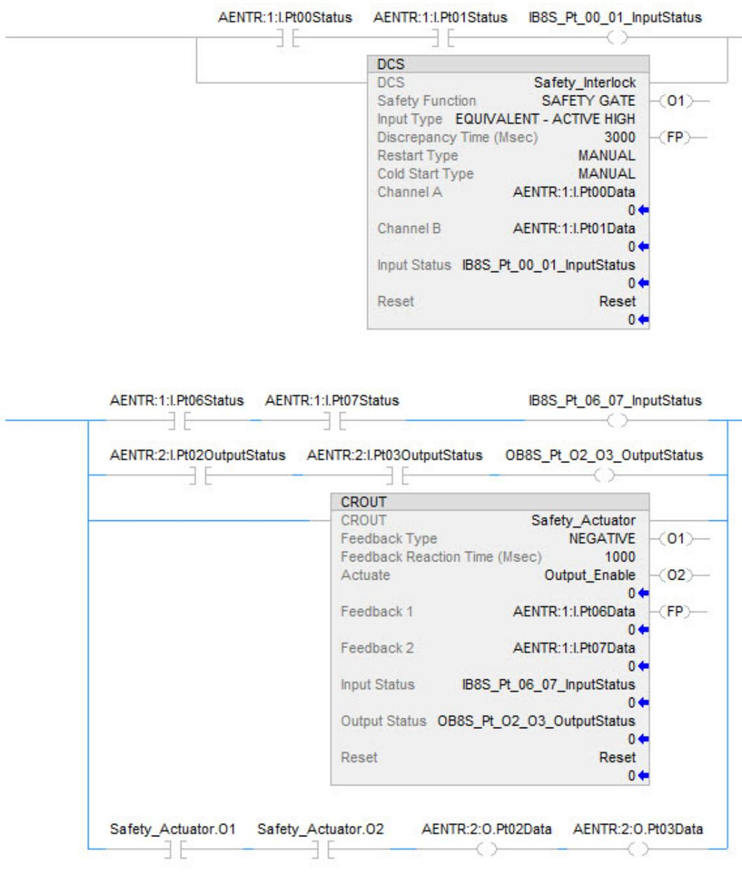
Safety I/O status should be interrogated when using instructions such as XIC and OTE. The responsibility for this falls to the user. You should verify that safety input channel status is HI (1) before using a safety input channel as an interlock. You should verify that safety output channel status is HI (1) before energizing a safety output channel.
