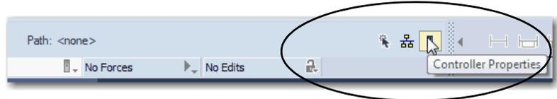
2. On the Controller Properties dialog box, click the Port Configuration tab.
