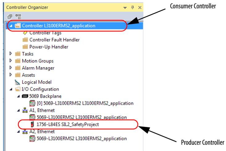
2. In the producer controller project, right-click the producer controller and choose Controller Properties.
