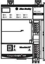
MOD power is a DC power source that is required to operate a CompactLogix 5380 system.
