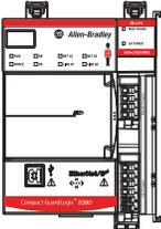
Slots of a Compact GuardLogix 5380 system chassis that are not used by the safety function can be populated with other Compact 5000™ I/O modules that are certified to the Low Voltage and EMC Directives. See <http://www.rockwellautomation.com/rockwellautomation/certification/cc.page> to find the CE certificate for the CompactLogix Product Family and determine the modules that are certified.
