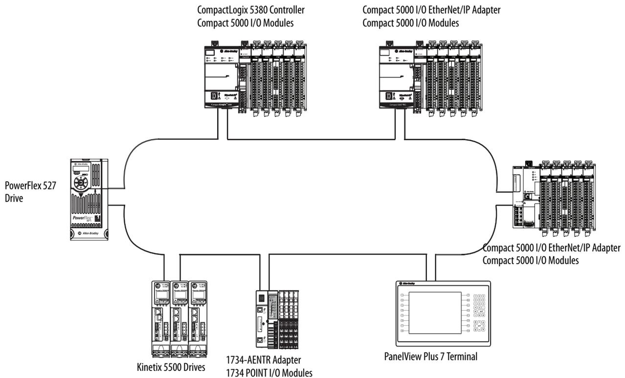
**Figure 28 - Compact GuardLogix 5380 Controller in Linear/DLR Mode in a Linear Network**
