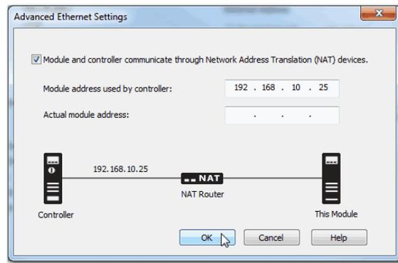
3. Check the checkbox to indicate that this module and the controller communicate through NAT devices.
