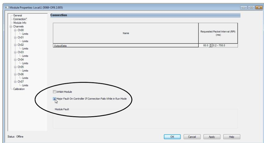
You can configure the application so that a response to a failed I/O module connection can wait until the next program scan. In this case, put the logic in a normal routine and use the GSV technique that is described on [page 237](#) to call the logic.
