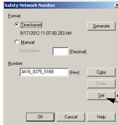
9. Verify that the Network Status (NS) status indicator is alternating red/green on the correct device before clicking Yes on the confirmation dialog box to set the SNN and accept the replacement device.
