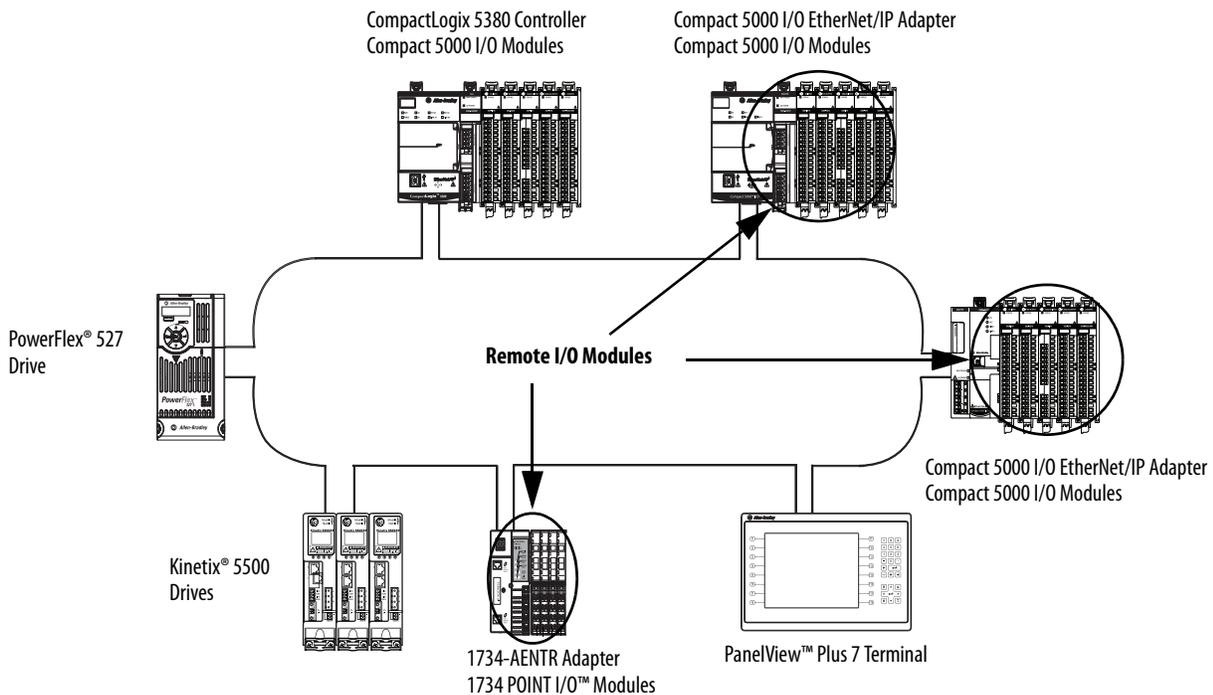
Figure 33 - Remote I/O Modules in a CompactLogix 5380 System on a Linear Network Topology
