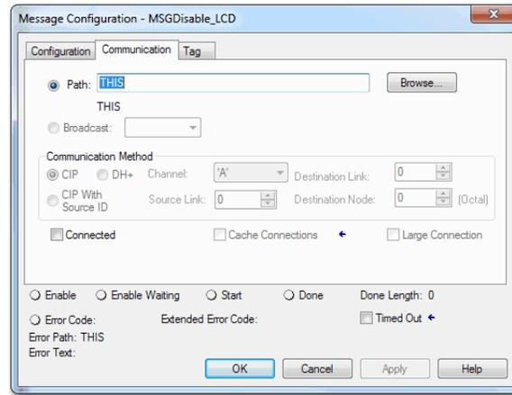
4. Before you enable the MSG instruction, make sure that the Source Element tag value is 1.
