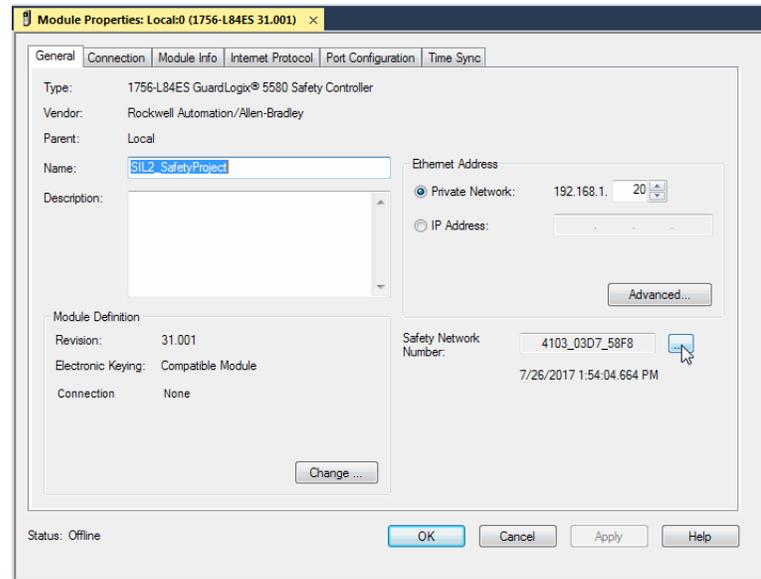
7. Paste the producer controller SNN into the SNN field and click OK.
