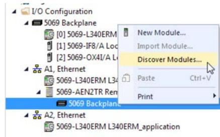
The Logix Designer application automatically detects available modules that are installed in the system.
