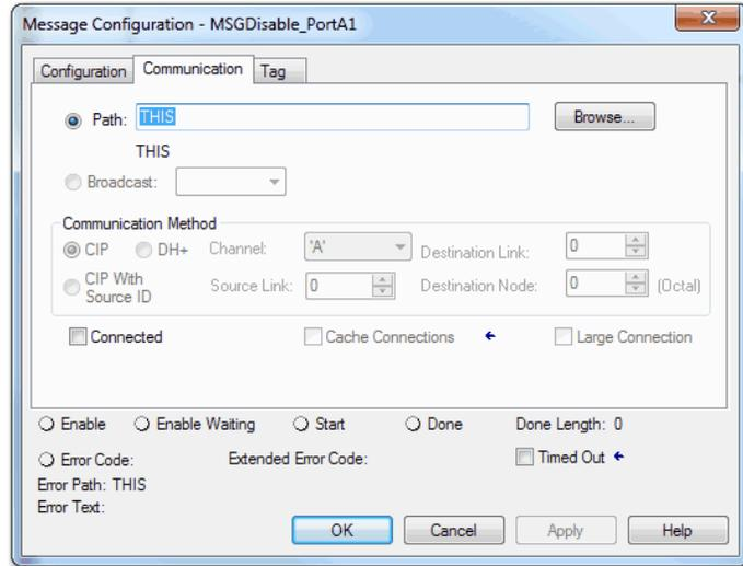
4. Before you enable the MSG instruction, make sure that the Source Element tag value is 2.
