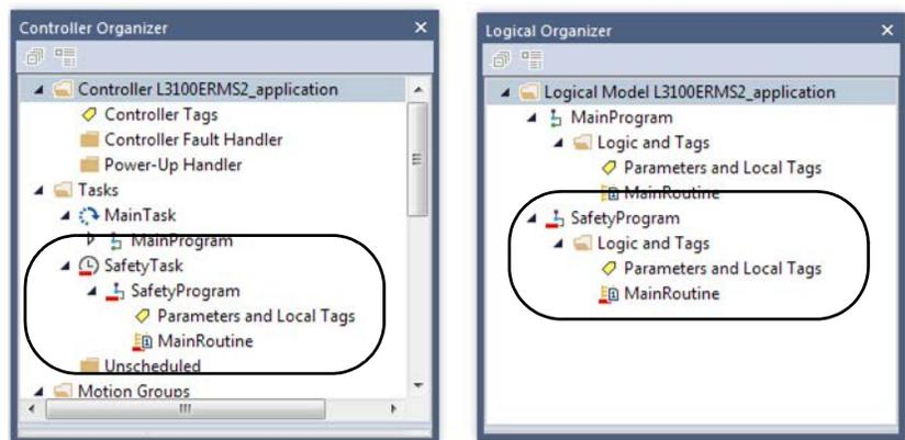
Within the safety task, you can use multiple safety programs, which are composed of multiple safety routines. The Compact GuardLogix® 5380 controllers support one safety task. The safety task cannot be deleted.
