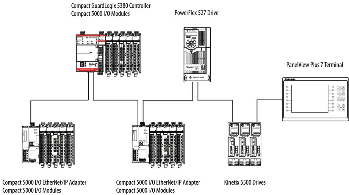
**Figure 29 - CompactLogix 5380 Controller in Linear/DLR Mode in a Star Network**
