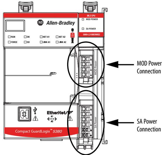
Power begins at the controller and passes across the Compact 5000 I/O module internal circuitry via power buses.
