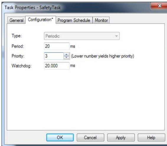
To get the most consistent safety task execution time, and to minimize safety task watchdog faults, we recommend running the safety task as the highest priority user task.
