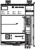
SA power provides power to devices that are connected to some of the Compact 5000 I/O modules in the CompactLogix 5380 system. SA power is connected to the controller via an SA power RTB.
