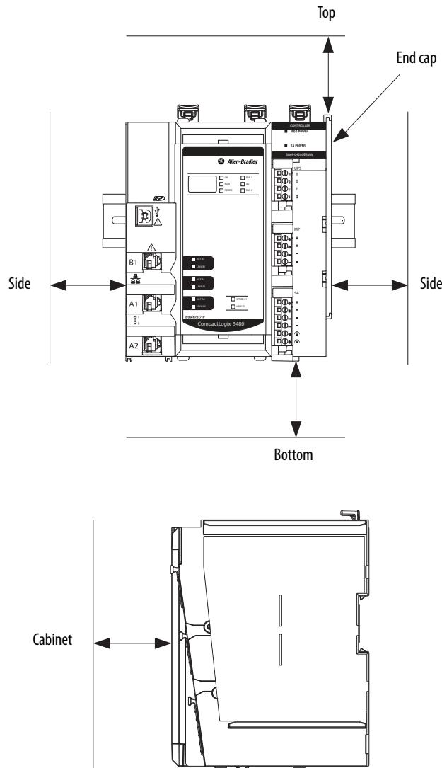
**IMPORTANT** If Compact 5000 I/O modules are installed next to a CompactLogix 5380, Compact GuardLogix 5380, or CompactLogix 5480 controller, you must mount the system horizontally.
